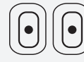
Left Button: Reticle brightness settings and On/Off button Right Button: Dot brightness settings and On/Off button
